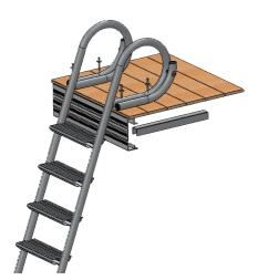
The Reinforcing Arm should be positioned so that it lines up with the holes of the Mounting Arm and should span as many decking boards as possible to spread the load. Secure in place with a clamp (or vice grips) and drill into the Reinforcing Arms while drilling the holes in the decking. To do this, you will need access under the decking so a deck board or two may need to be removed during installation.
